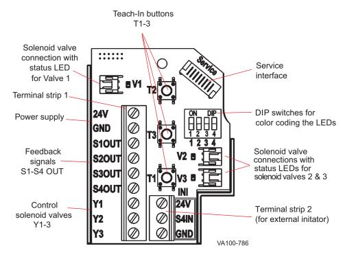
Figure 37 - 24 V DC Electronics Module Terminal Strip Configuration
