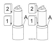
Figure 64 - Valve Closed Adjustment
