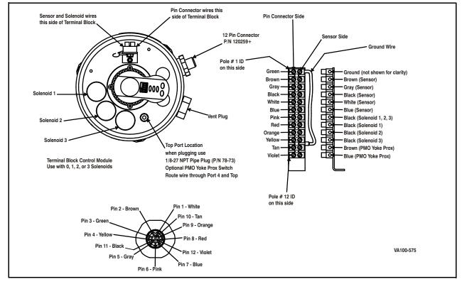
Figure 13 - 12-pin Eurofast wiring
