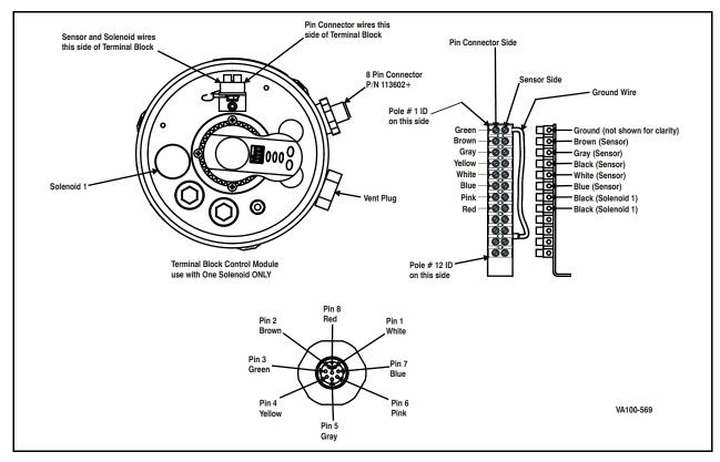
Figure 11 - 8-pin Eurofast wiring
