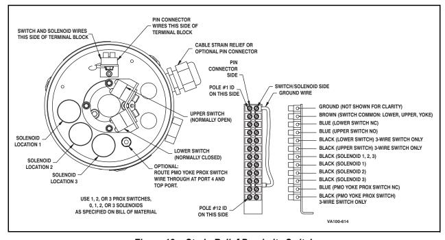
Figure 18 - Strain Relief Proximity Switch
