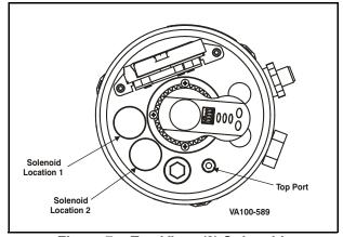
Figure 7 - Top View, (2) Solenoids
