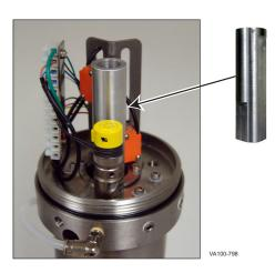
Figure 65 - Quick-set Proximity Switch Gauge
