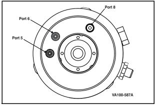
Figure 4 - Control Top Bottom View, Ports 5,6,8
