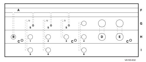
B.Air-In C.Setscrew D.Vent E.Wire F.Inside Diameter View G.Top View H.Side View I.Underside View S.Solenoid Mount
