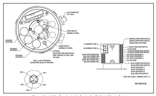
Figure 22 - 5-Pin Eurofast with DeviceNet™ Card, Single Seat
