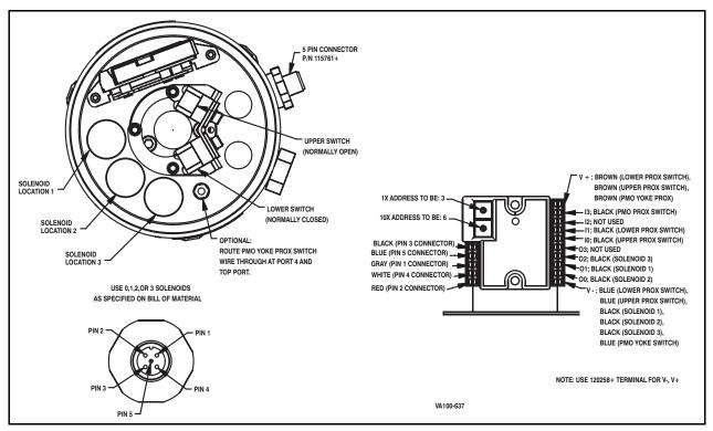
Figure 23 - 5-Pin Eurofast with DeviceNet™ Card, Mix Proof
