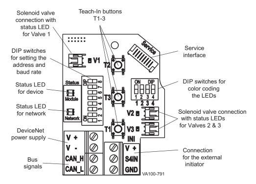
Figure 42 - DeviceNet™ electronics module
