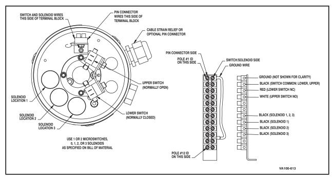
Figure 17 - Strain Relief Micro Switch
