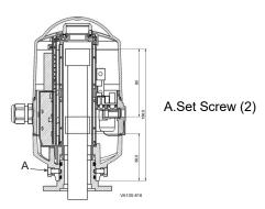
Figure 49 - Bürkert Control Top Removal
