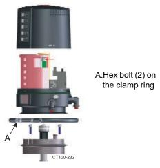
Figure 50 - CU4 Control Top Removal
