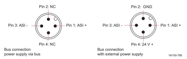
Figure 39 - AS-interface® bus connection (power supply via bus / external power supply)
