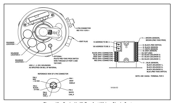
Figure 15 - DeviceNet™ Eurofast Wiring, Single-Seat
