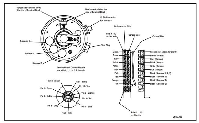
Figure 12 - 10-pin Eurofast wiring
