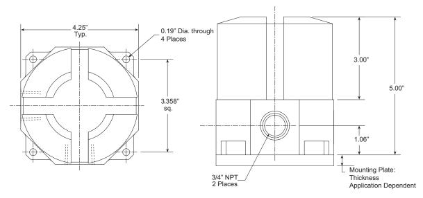
Figure 46 - Explosion Proof Westlock/Tyco Control Top Dimensions
