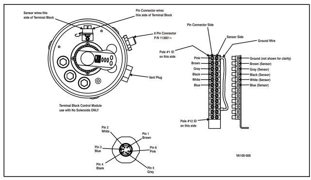
Figure 10 - 6-pin Eurofast wiring
