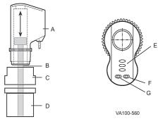
A.Sensor B.Stem and Target C.Sensor Mount D.Actuator E.3 LEDs Open, Seat, Close F. Teach Button G.Pos. Button
