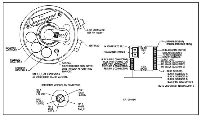
Figure 16 - DeviceNet™ Eurofast Wiring, Mix Proof
