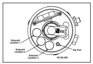
Figure 8 - Top View, (3) Solenoids
