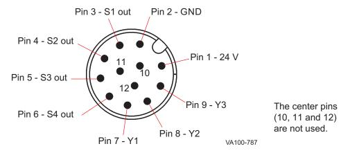
Figure 38 - 12-pole multi-pole connection
