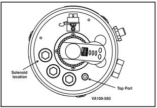
Figure 5 - Top View, No Solenoids
