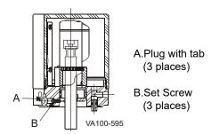
Figure 48 - WCB Control Top Removal
