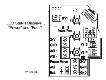
Figure 40 - AS-interface<sup>®</sup> Electronics Module - LED Status Displays
